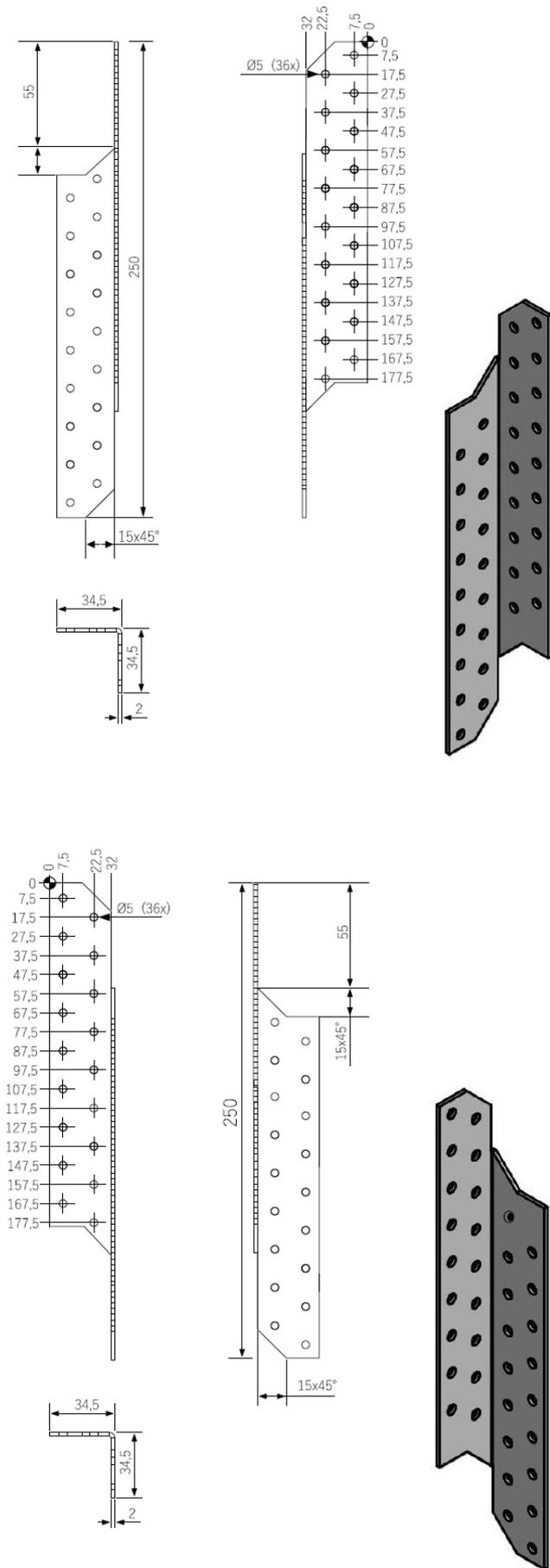
Figure A.3 Dimensions of Purlin Ties 250 right/left
