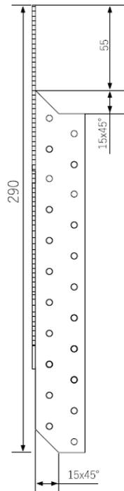
Figure A.4 Dimensions of Purlin Ties 290 right/left
