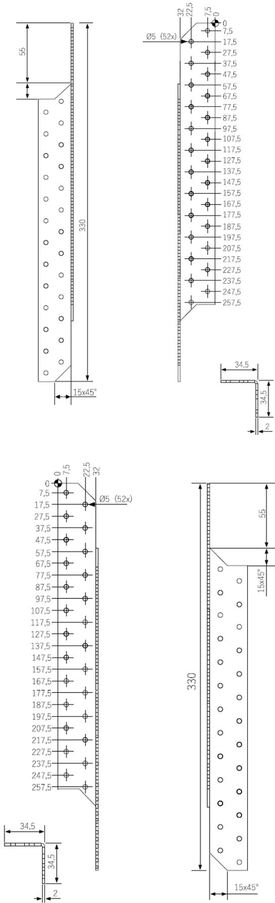
Figure A.5 Dimensions of Purlin Ties 330 right/left
