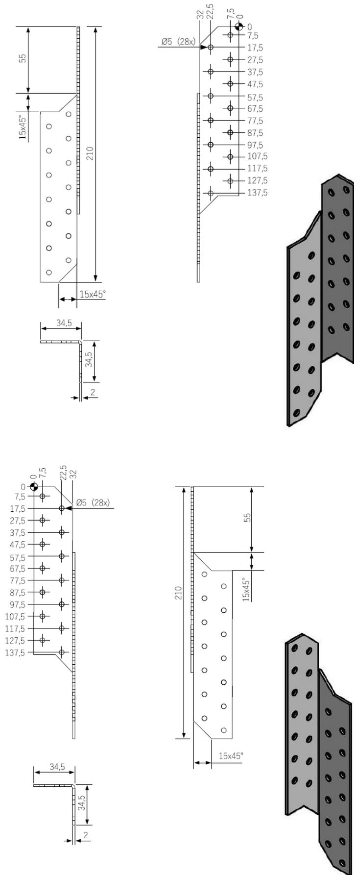
Figure A.2 Dimensions of Purlin Ties 210 right/left
