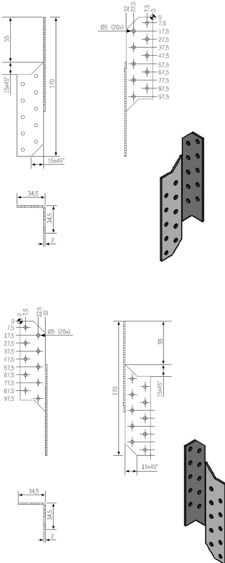
Figure A.1 Dimensions of Purlin Ties 170 right/left
