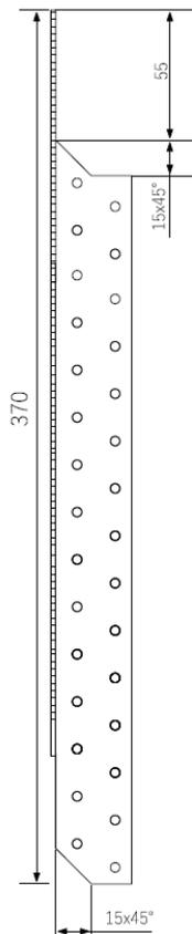
Figure A.6 Dimensions of Purlin Ties 370 right/left
