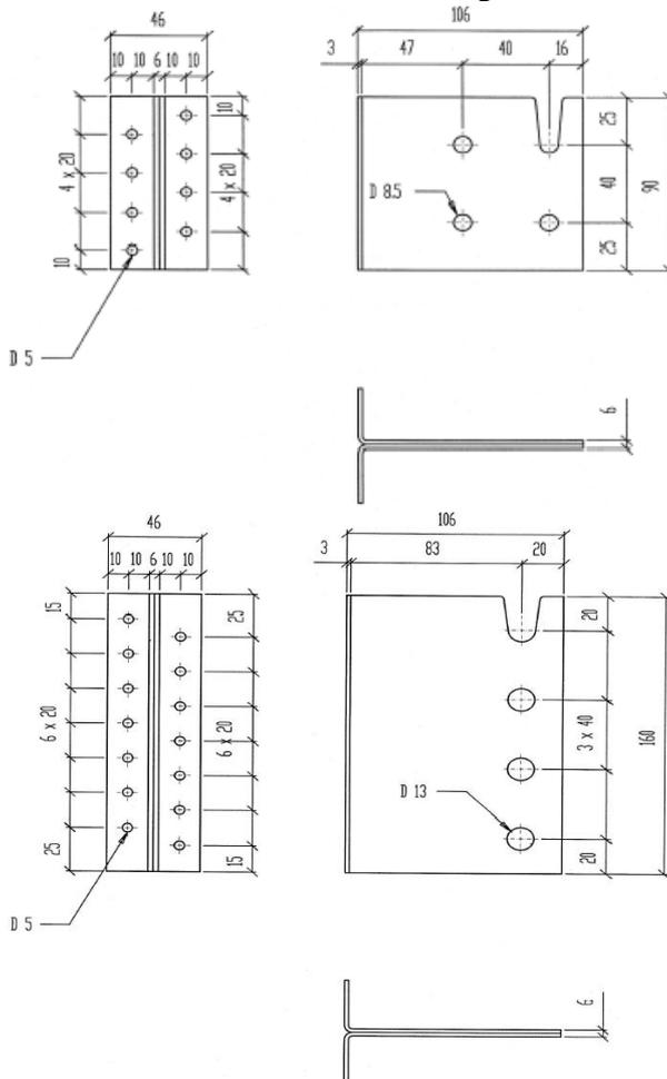
Drawing: beam hanger 90 (left), beam hanger 160 (right)
