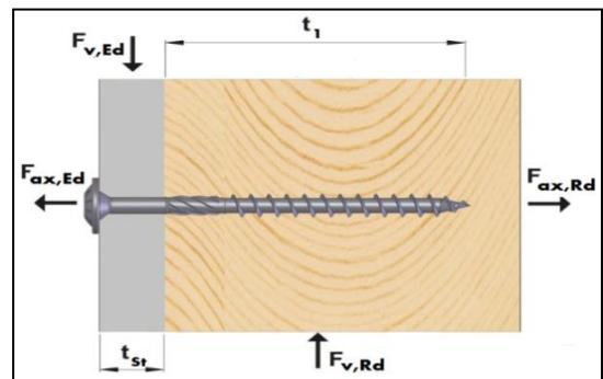
Axial tensile strength  $F_{ax,Rk}$  or  $F_{ax,Rd}$       Shear strength  $F_{v,Rk}$  or  $F_{v,Rd}$
