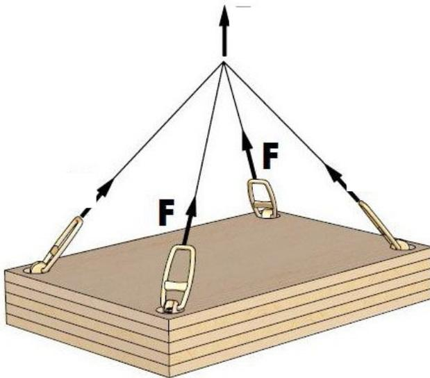
Statically undefined suspension gear ( $n = 2$ )
