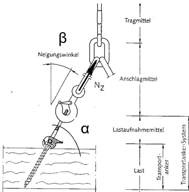
Transport anchor under axial tensile load
