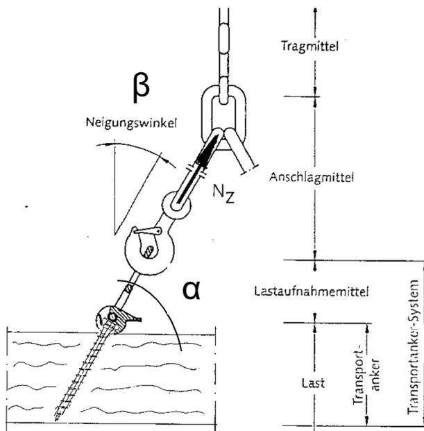
Transport anchor under axial tensile load
