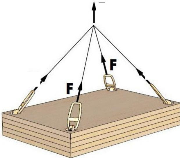
**Statically undefined suspension gear (n = 2)**
