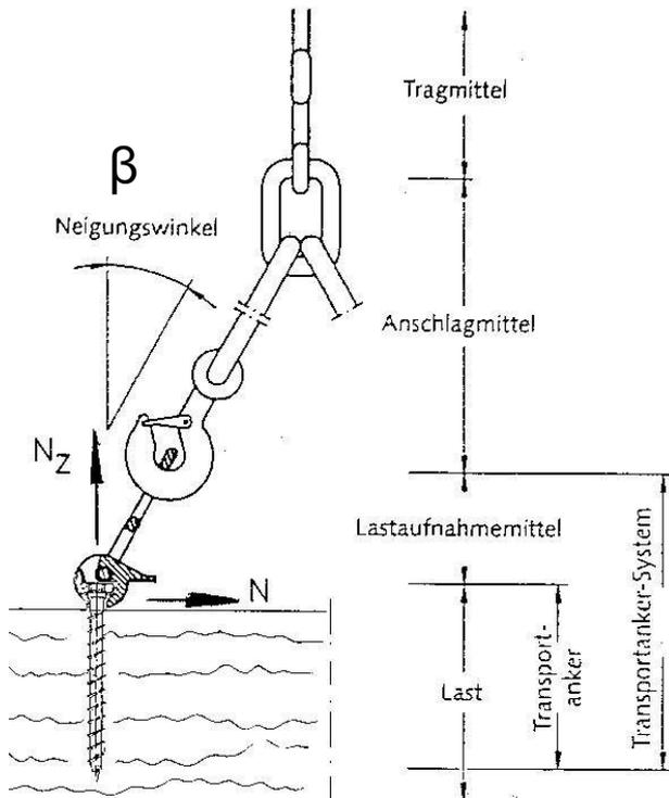
**Transport anchor under inclined load**
