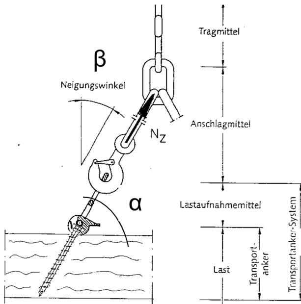
Transport anchor under axial tensile load
