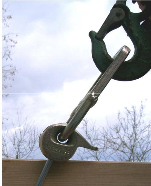
**Transport anchor system with the ASSY 4 Combi T self-tapping screw and DEHA universal coupling, load group 1-1.3**
