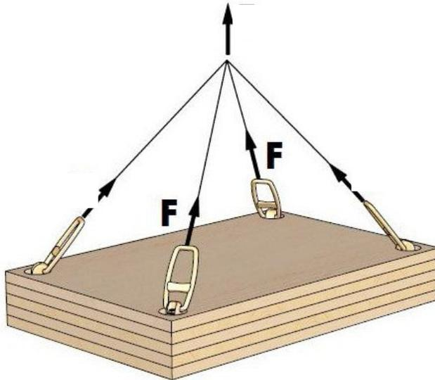
**Statically undefined suspension gear (n = 2)**
