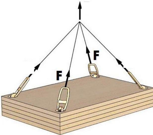
**Statically undefined suspension gear (n = 2)**
