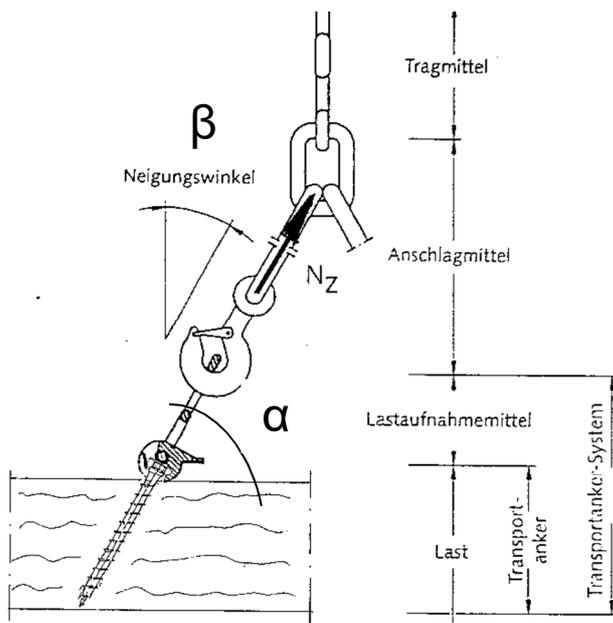
**Transport anchor under axial tensile load**
